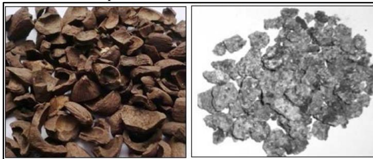
Fig. 4 OPS and POC aggregate used by Md. Nazmul, et. al, 2016
